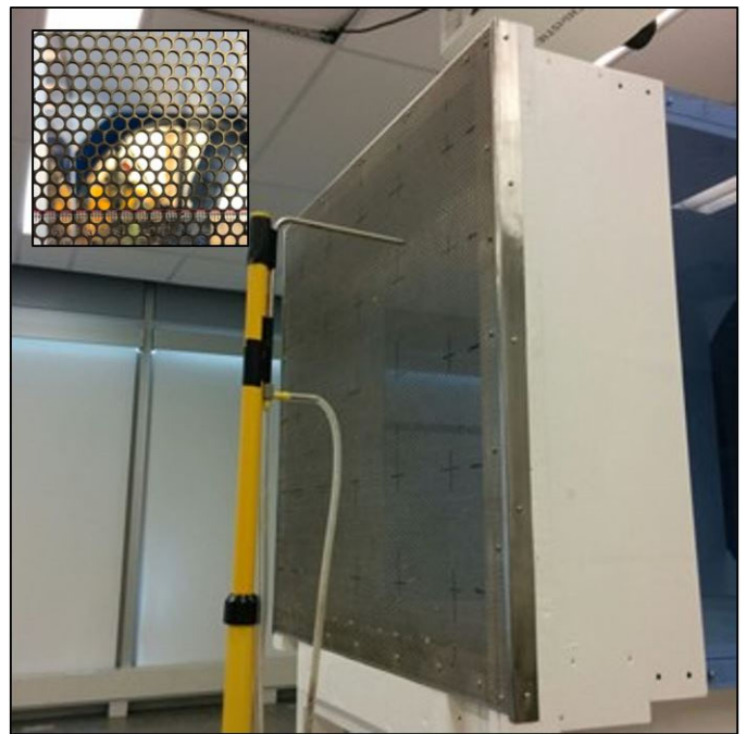
Figure 2. Fan outlet diffuser grid with pitot probe
