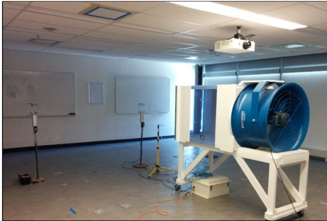
Figure 1. Fan positioned in room and sonic anemometers
